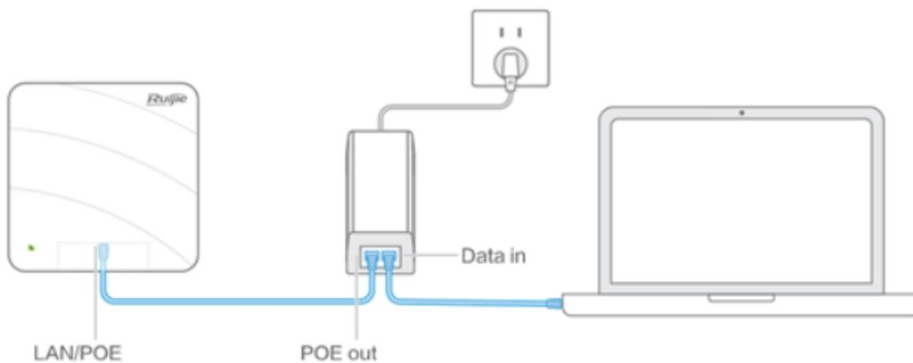
2. POE switch power supply connection diagram.
